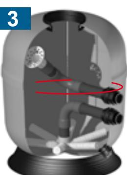
Pour the sand (granulometry 0.6/1.25) in carefully to avoid damaging the laterals.
