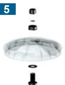
Assemble the air bleed valve on the lid.
