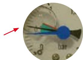
After a certain time, a drop in the flow rate may be noted at the return fittings. This is caused by the gradual build up of impurities in the filter or the filter basket.
