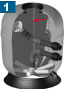
Remove the diffuser and swing the collector to the side.
