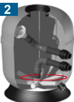
Check that the drain valve is closed.
