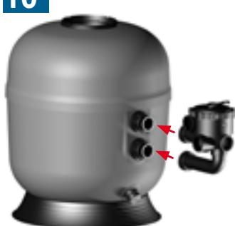
Mount the multi-port valve. Connect the lower bulkhead fitting and then the upper bulkhead fitting. Tighten the nuts moderately.
