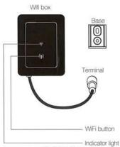
Green:Network connection Orange:No network Red:Failure
