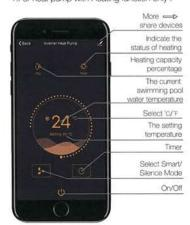
2. For heat pump with Heating&Cooling function:
